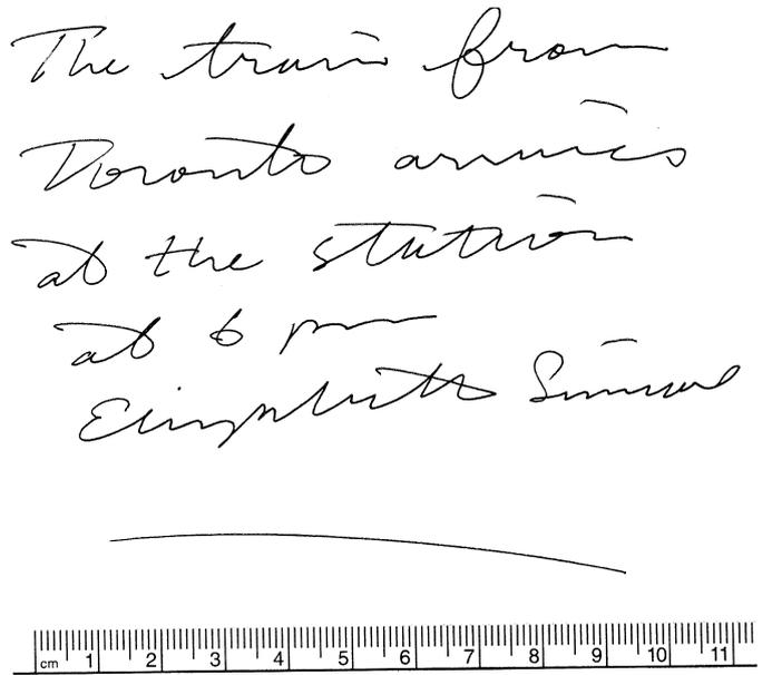
FIG. 5—Roller ball pen specimen written with the LongPen Kiosk, fast speed.
