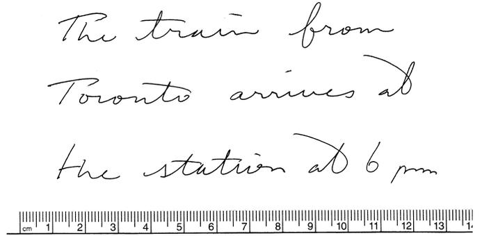
FIG. 3—Roller ball pen specimen written with the LongPen Kiosk, normal speed, normal pen pressure.
